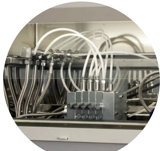
Dual extraction by pressure rinse and internal rinse
